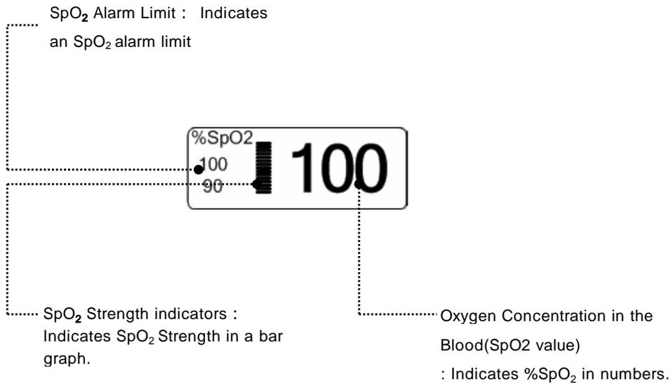
The current SPO2 value and the derived pulse rate (RATE) are displayed. The block sets indicate the strength of the signal (twenty block bars indicate the strongest signal). The SPO2 measurements are averaged over a 6-second period of time.
