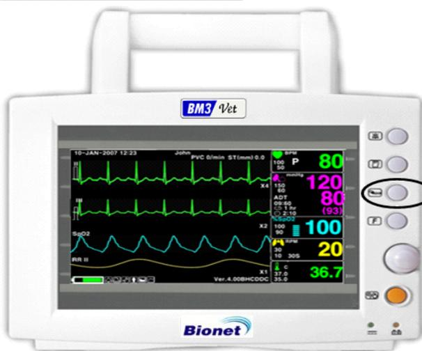
The manual press of external NIBP key can start or stop the operation of NIBP.
