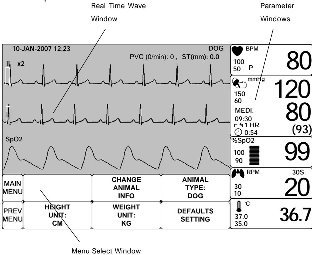
Real Time Wave Window : Displays measured results by up to three waves.
